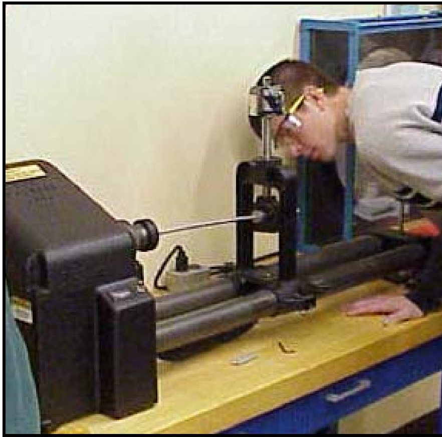
Figure 13: Fatigue Testing Equipment for Alternating Loading
