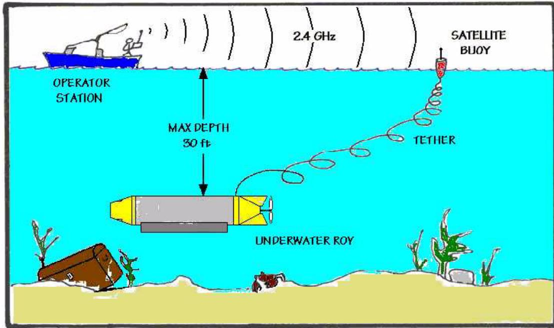
Figure 3. Schematic of ROV system.
