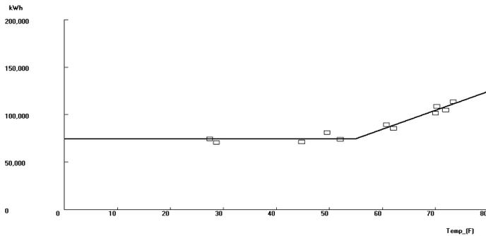
Figure 3. Linear Regression Analysis of Facility Electric Use
