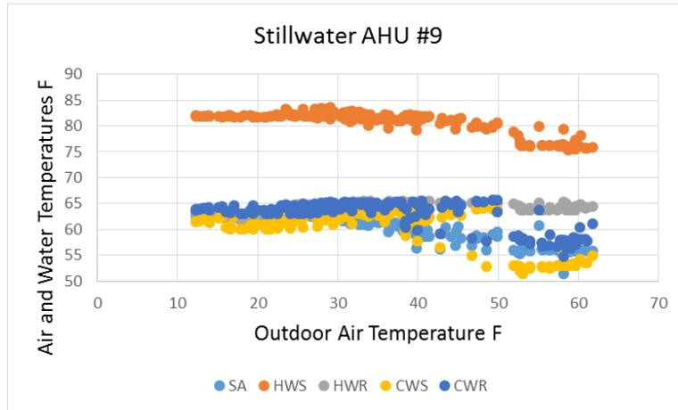
Figure 10. Supply Air Temperature, Hot and Cold Supply and Return Water Temperatures, Example of Analysis of HVAC Data Logging
