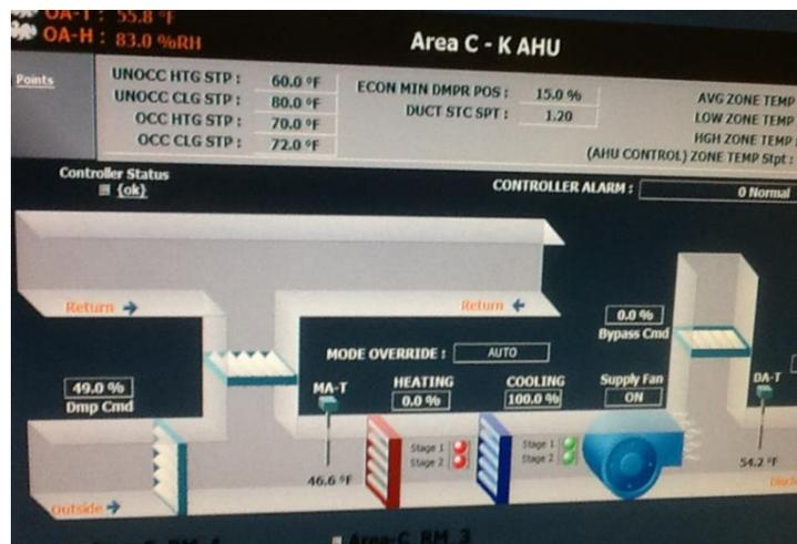
Figure 6. Screen Copy of Building Automation System
