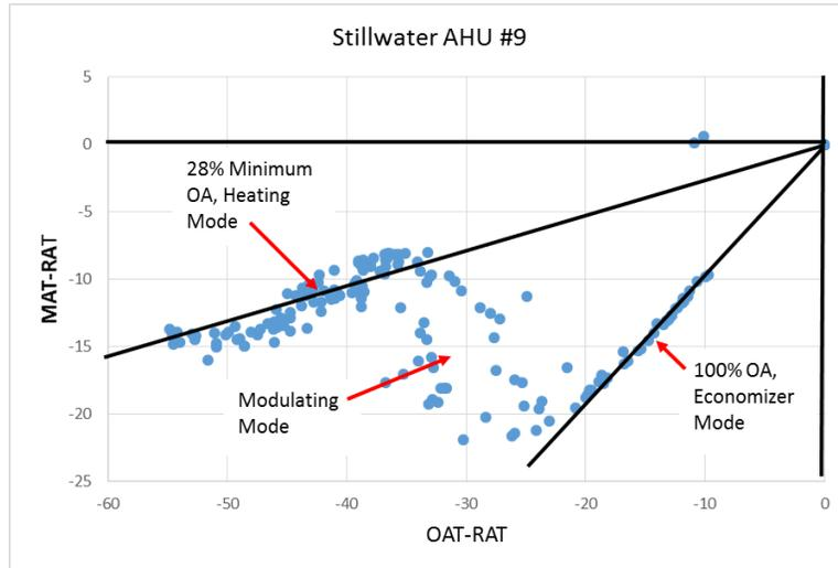
Figure 7. Mixed Air Temperature – Return Air Temperature Plotted over Outdoor Air Temperature – Return Air Temperature
