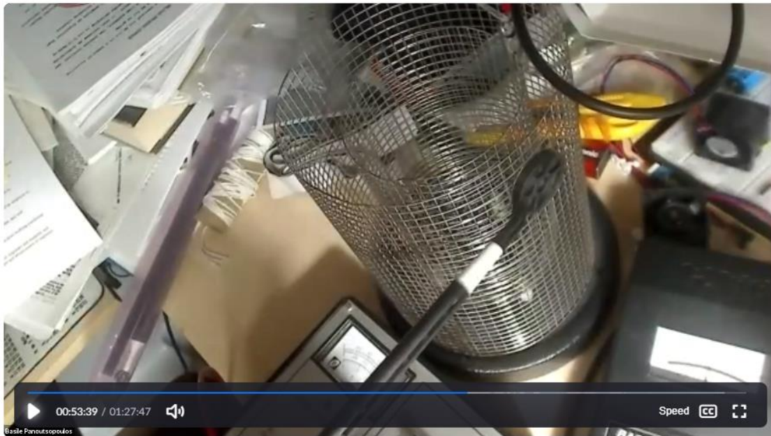
Figure 03. Experimental setup of a remote learning experiment (Gauss Law – Electric Charge Distribution). Grounding of the proof plane.
