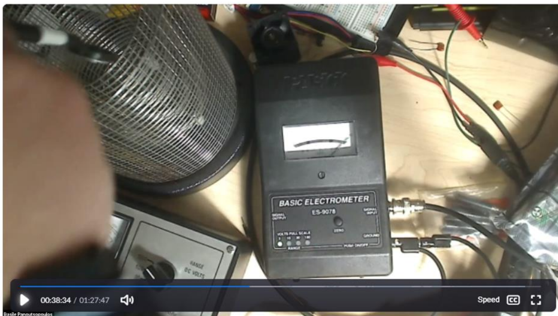
Figure 04. Experimental setup of a remote learning experiment (Gauss Law – Electric Charge Distribution). Measurement of electric charge.
