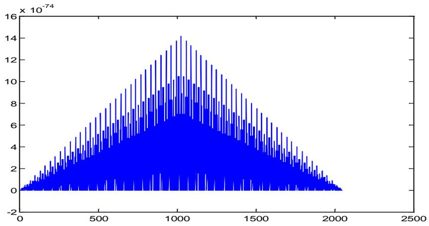
**Figure 3** Autocorrelation of Received signal in UWC channel
