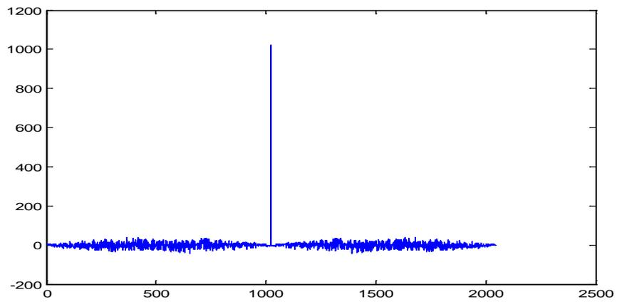
**Figure 2** Autocorrelation of single transmitted m-sequence
