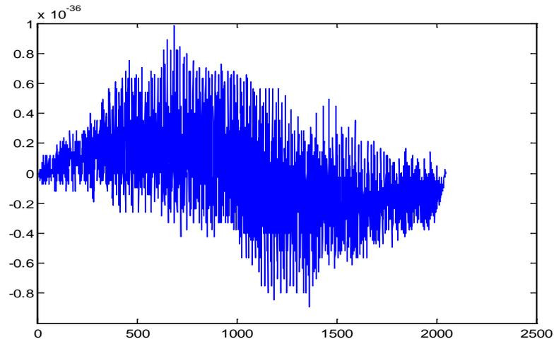
**Figure 1** Cross correlation between Transmitted signal and Received signal for UWC channel
