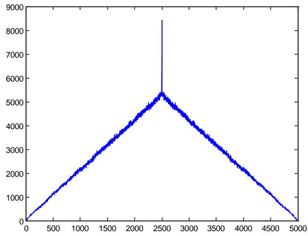
**Figure 5** Simulated result for cross correlation of transmitted and received signal for ideal channel
