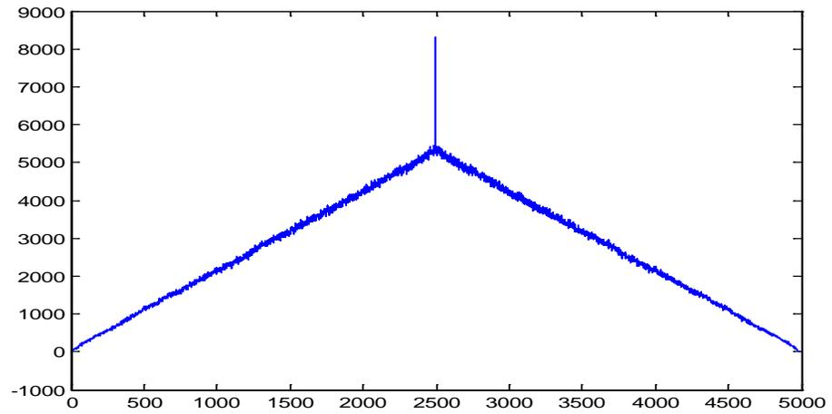
**Figure 4** Simulation result for autocorrelation of random integers transmitted in ideal channel
