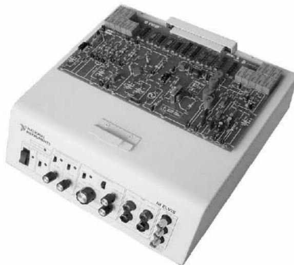
Figure 3 eTCB board interfaced with NI ELVIS workstation 13
