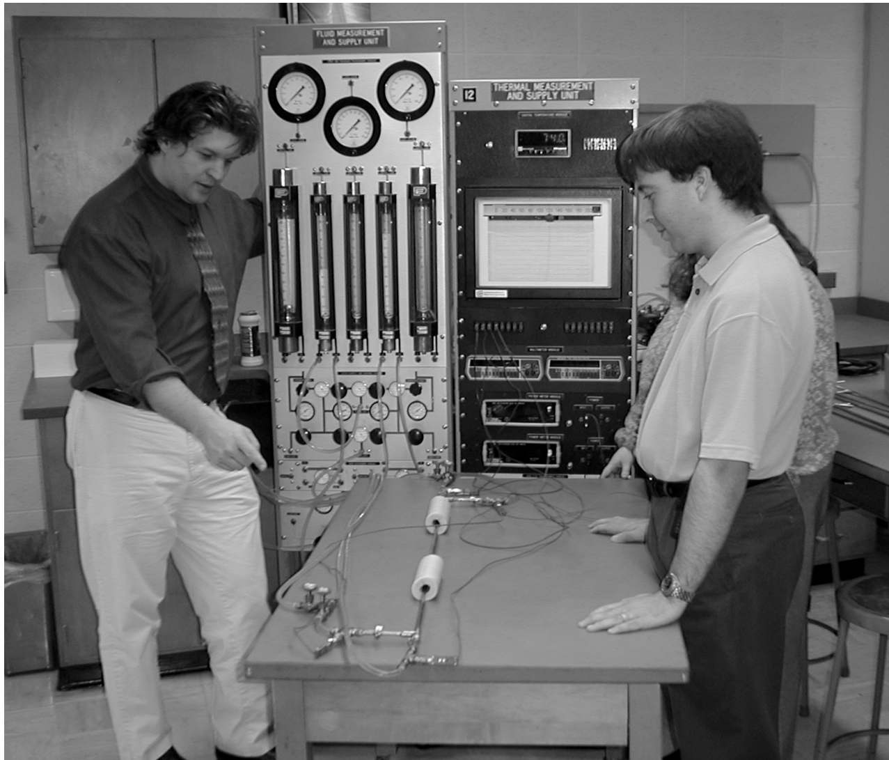
Figure 8. Testing of the heat exchanger.
