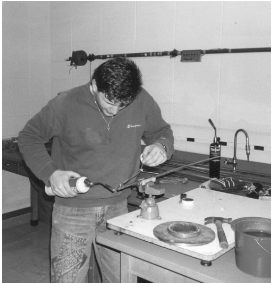
Figure 6. Sweat Soldering of the Thermal Recuperator.
