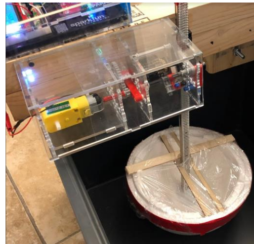
Fig. 4. Photograph of the wave energy converter.
