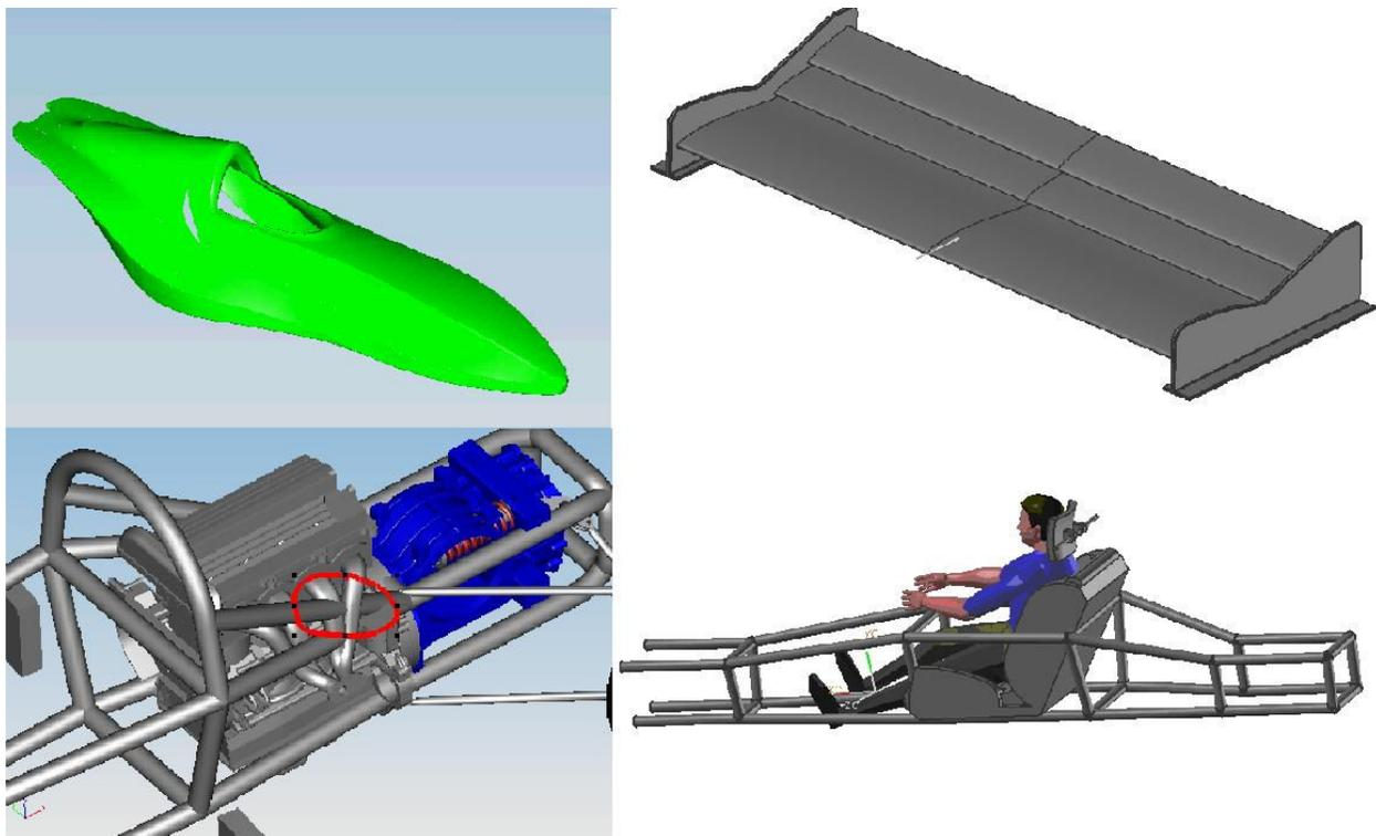
**Figure 6:** Pictures such as these were used to quickly and effectively communicate design intent to solve problems and continue on with design iteration. From the top left: 1) the Korean university's finished body model, 2) the Swedish university's wing mounted in the Australian university's mounting bracket, 3) the frame-engine interference issue highlighted in Teamcenter visualization, and 4) the Korean university's original seat in the American university's frame.
