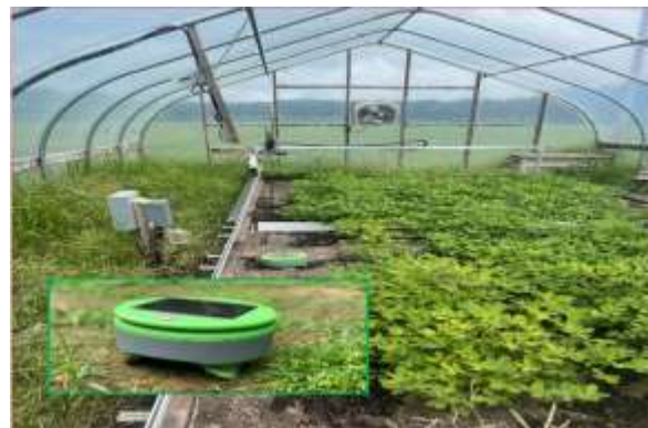
Figure 1b: View from inside the high tunnel with a inset of a solar powered robotic weeder
