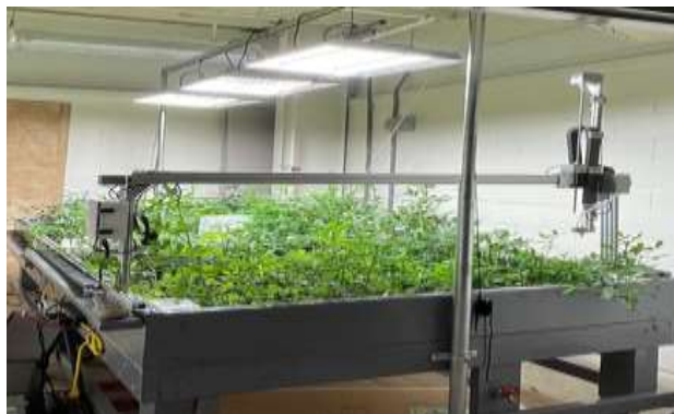
Figure 2a : Indoor FarmBot with Growlights, the Farmbot bed is on a mobile table
