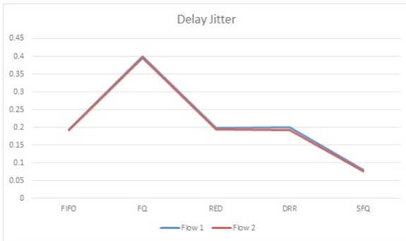
Fig. 7. Graph shows delay jitter of each flow.
