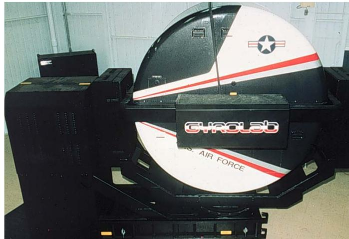
Figure 6. Motion based flight simulator.
