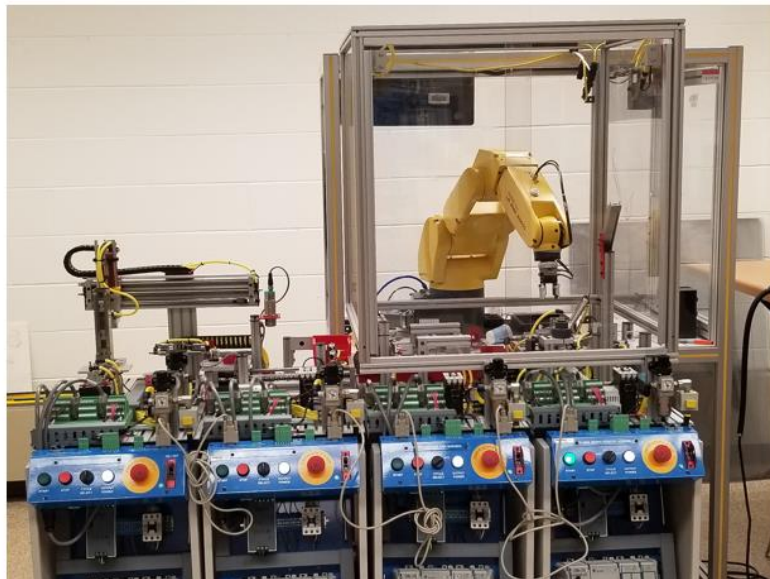
Figure 7: SoT Robotics Lab – Mechatronics assembly line retrofitted with FANUC LR 200iC industrial Robot
