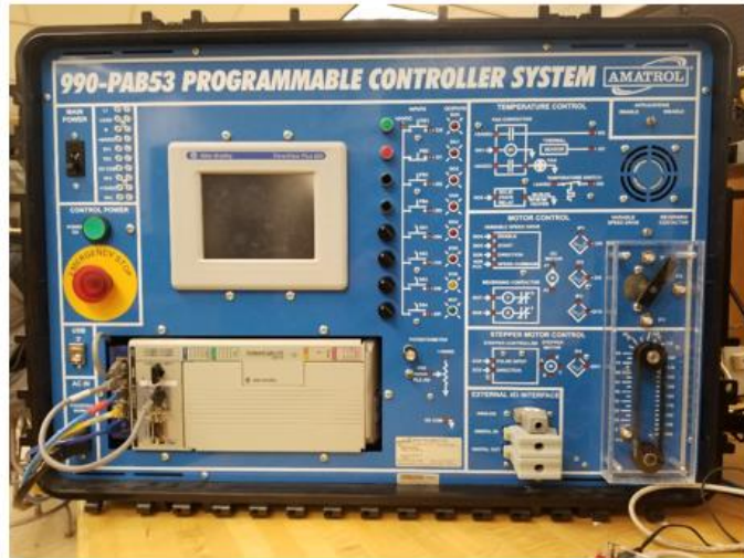
Figure 8 (a): SoT and ECE PLC Lab – Amatrol 990PAB53 Portable PLC Learning Systems
