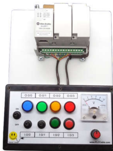
Figure 4. An Allen-Bradley Micro 820 trainer used for the final project of the PLC module.
