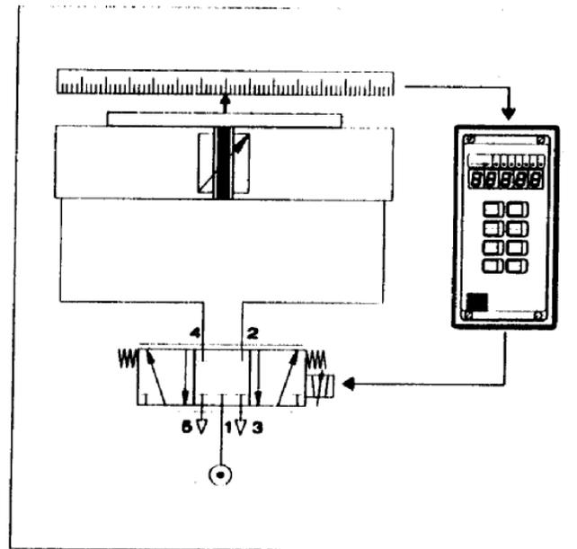
Figure 2. Structure of a positioning control circuit with pneumatic components
