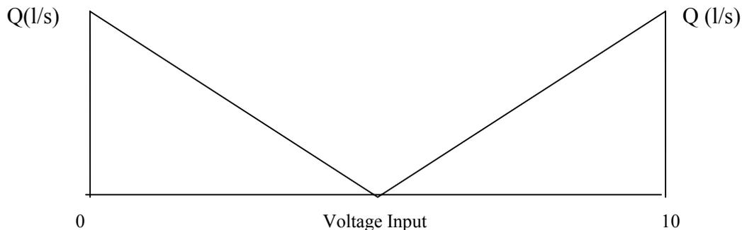
*Figure 4. Schematic of the MPYE Proportional Servo Valve*
