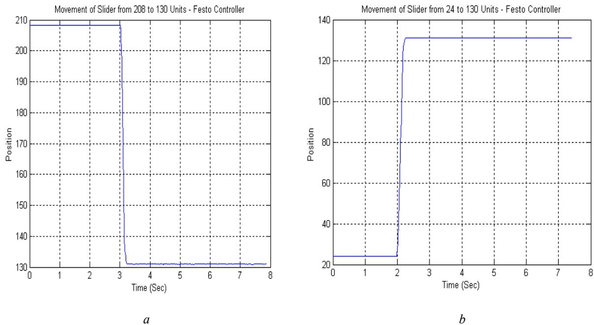
*Figure 3. Position response of SPC 100 Controller*
