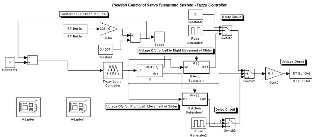
Figure 7. Simulink™ Model for Servo Pneumatic System using Fuzzy Control
