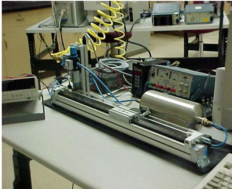
*Figure 1. Festo™ Servo Pneumatic Actuator & Control System*
