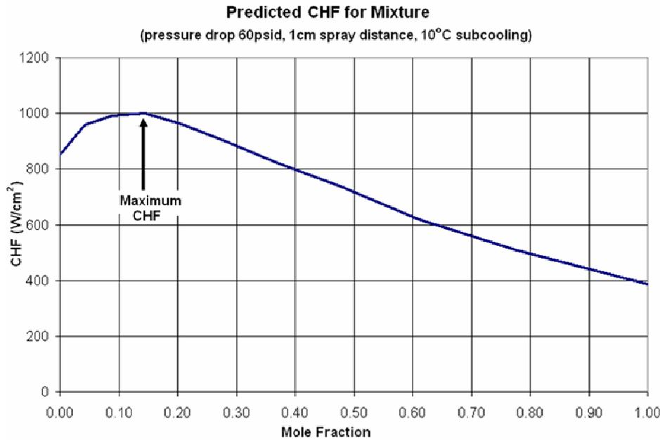
**Figure 2: Predicted Critical Heat Flux possible by a two-liquid mixture.**
