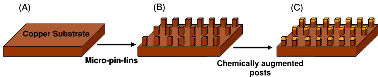
**Figure 1: Schematic of a (A) traditional copper substrate heat sink, (B) substrate with micro-pin-fins machined into surface, and (C) final augmented design with chemically enhanced posts.**
