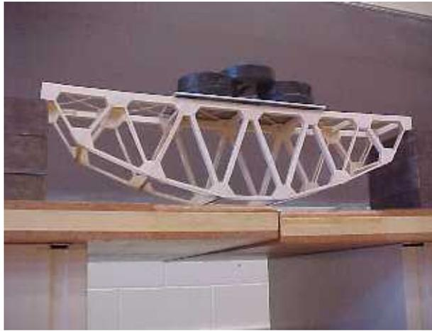
*Figure 3: Bowstring Deck Truss made of Manila File Folder<sup>13</sup>*
