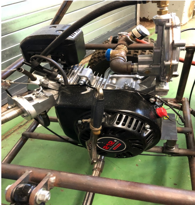
Figure (3) One-cylinder Gasoline engine Predator 212cc engine conversion kit
