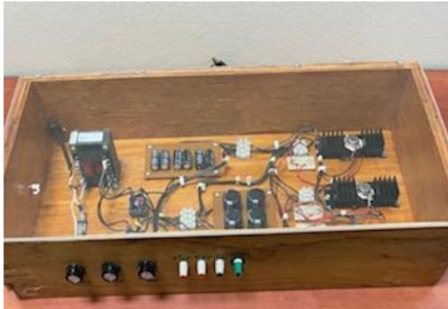
Figure 7: Student power supply enclosure design: example 6
