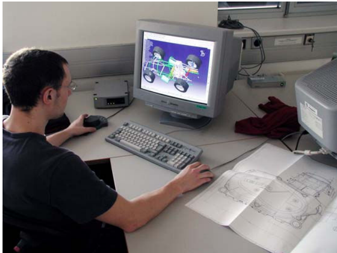
Figure 12: Designing the racing car with CATIA V5
