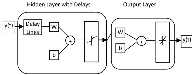
Fig. 3. Neural network architecture for the predictive model. The network is a two-layer feedforward network, with a sigmoid transfer function in the hidden layer and a linear transfer function in the output layer. This network also uses tapped delay lines to store previous values of  $y(t)$  sequences.  $W$  is the weight matrix, and  $b$  is the bias.
