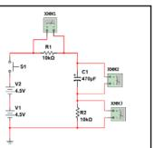
**2c) RC Circuit Transient Analysis** – Put a 100 $\mu$ F in parallel with the 470  $\mu$ F capacitor and repeat part 2b.
