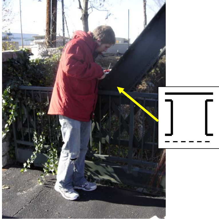
Figure 4: Student Measuring Section Properties of a Truss Diagonal
