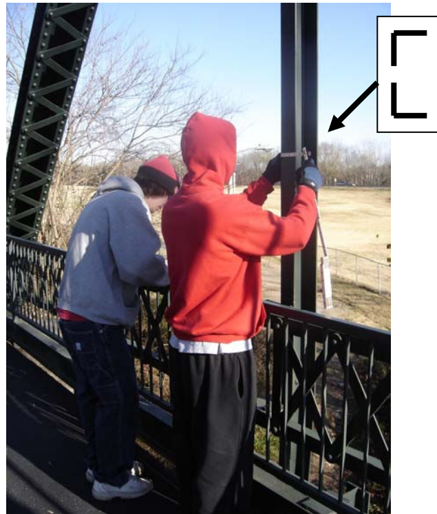
Figure 3: Students Measuring Section Properties of a Vertical Truss Member.
