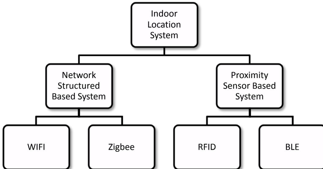
**Figure 2:** Methods and technologies for indoor location.
