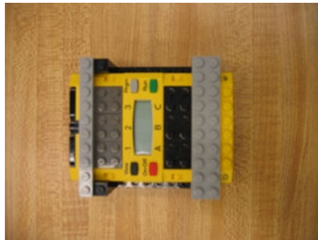
Figure 7: Structure built around the RCX.
