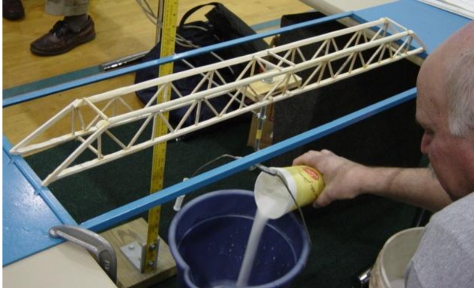
Fig 3. Model bridge being tested using a block of wood, threaded hook, and glass beads being slowly poured into the bucket.
