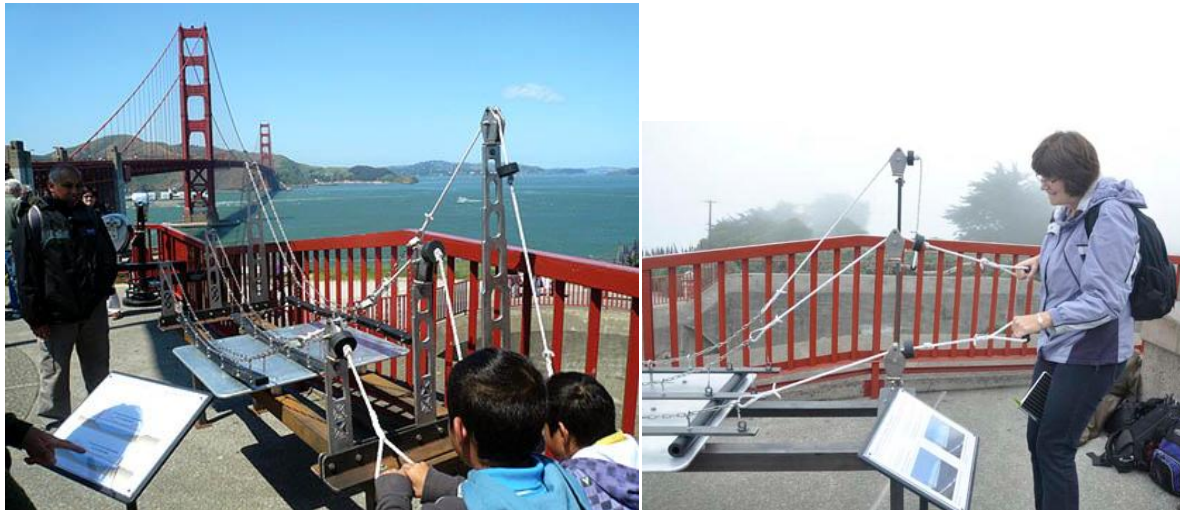
Figure 5. Visitors pull on the main cable to discover that the cable force is larger when the sag is less. (credit: R. Reitherman)
