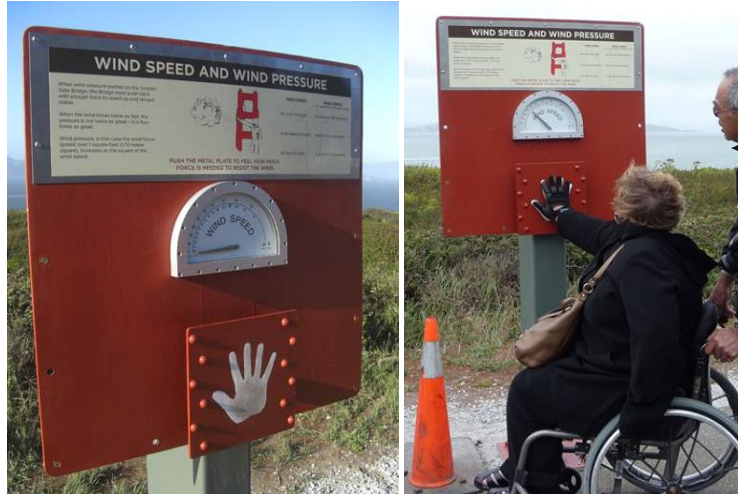
Figure 10. Visitors push on the display to experience the forces the bridge must supply to resist the wind pressure. (credit: R. Reitherman)
