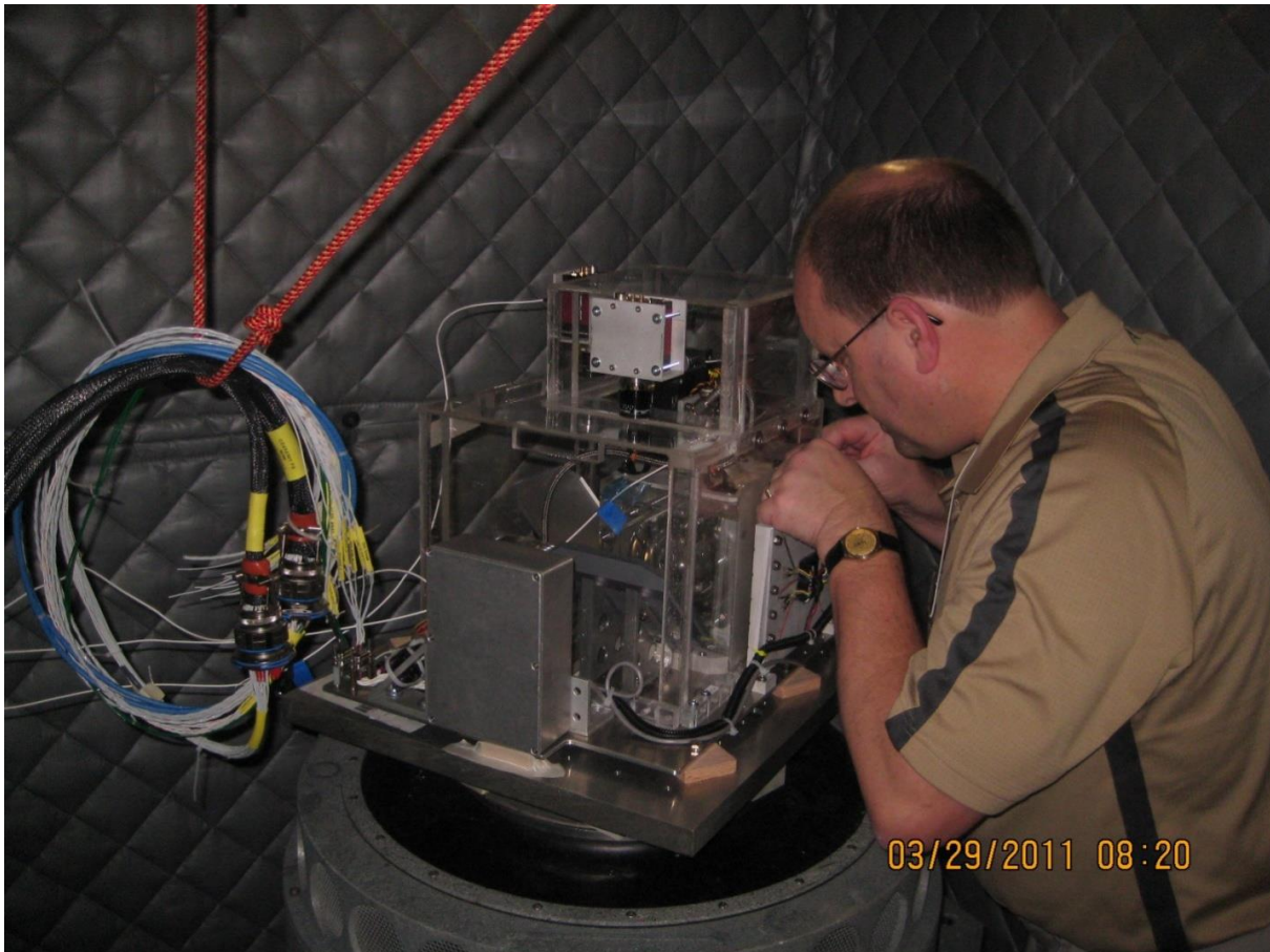
Figure 4. Blue Origin payload on a vibration test table prior to the successful vibration test. Final preparations being made by the author.
