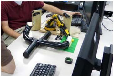
Figure 3 Workstation with ball return. The robot was programmed to pick and place balls on either end of a return, demonstrating increased repeatability through the use of sensors. The sensors and robot motors were controlled using MATLAB.
