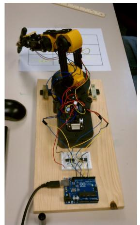
Figure 1 Assembled robot kit used in the Robotic Application version of the course. The computer is tethered by a USB cord to an Arduino Uno, which controls the robot motors.
