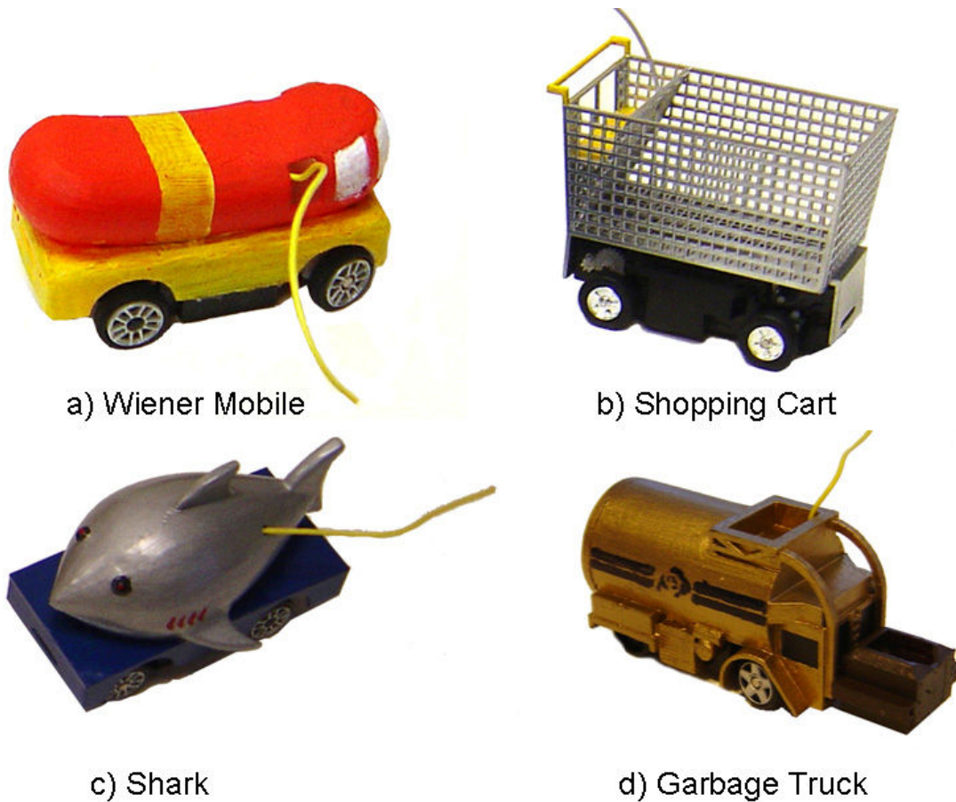
Figure 3. Example stereolithography (SLA) projects. The yellow wire is the radio control antenna.
