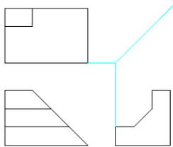
Figure 5.54.16 - finish the top view
