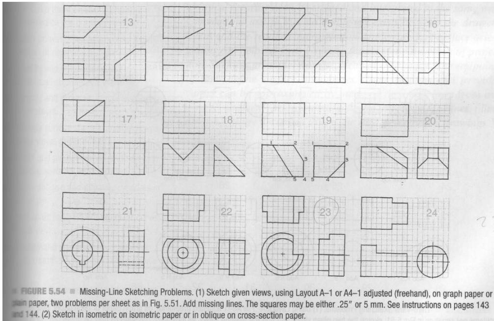
Figure 5.54 from text – completing unfinished view.
