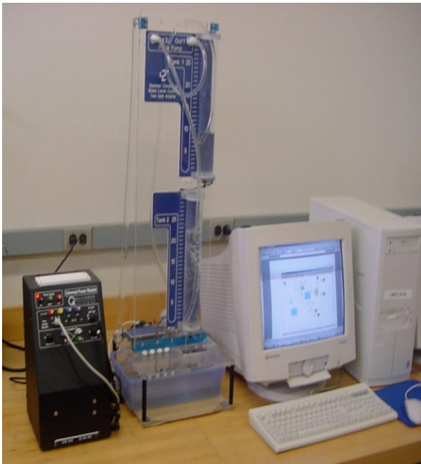
Photograph 3. Dual Water Tank System
