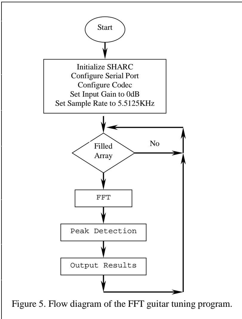
Figure 5. Flow diagram of the FFT guitar tuning program.
