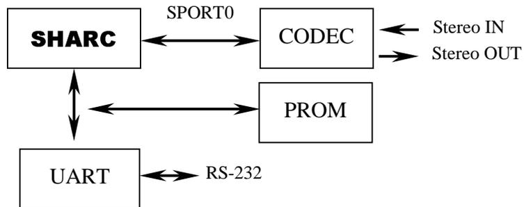
Figure 1. EZ-KIT Lite functional block diagram.
