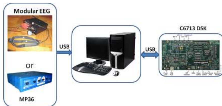
Figure 5 Connection of system hardware
