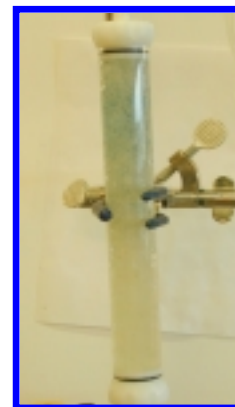
Figure 4. Immobilized enzymes in a continuous packed column reactor.
