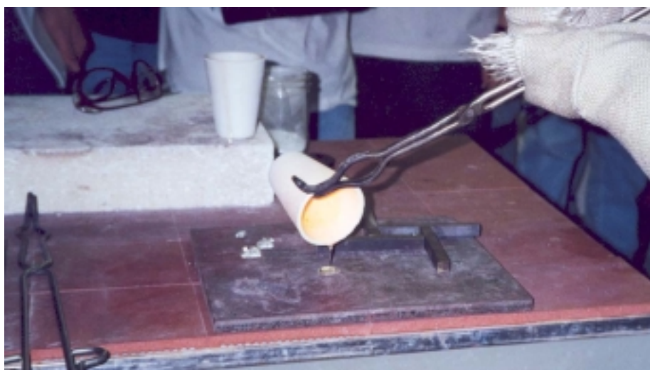
Figure 3. Pouring of a high temperature borate-based glass.
