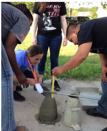
Students perform a slump test, 2015
