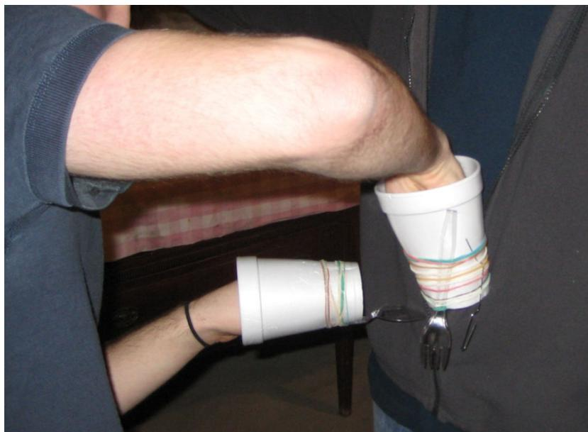
**Figure 1. Representative Prosthetic Hands Performing the Task of Zipping up a Jacket**
