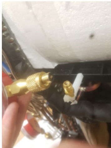
Figure 5. Quick disconnect connectors welded into the refrigerant pipes
