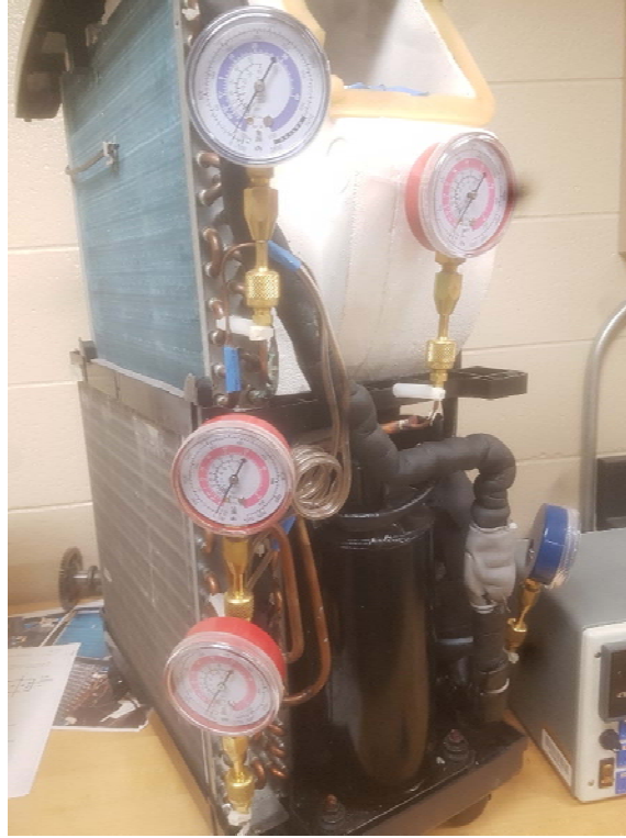
Figure 8. Pressure gages welded into the refrigerant pipes
