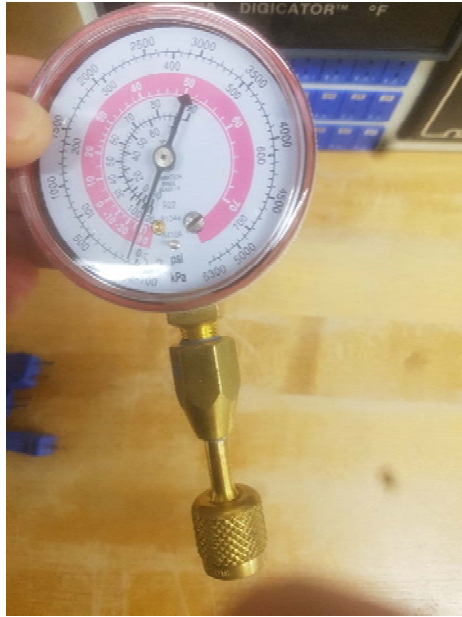
Figure 6. Pressure gage with quick disconnect welded into its inlet connection
