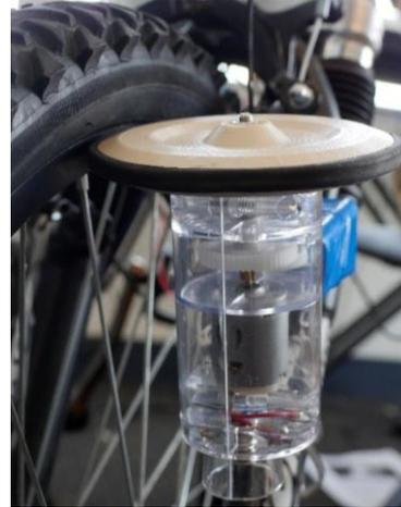
Figure 2b: RE-Brake on a bike
