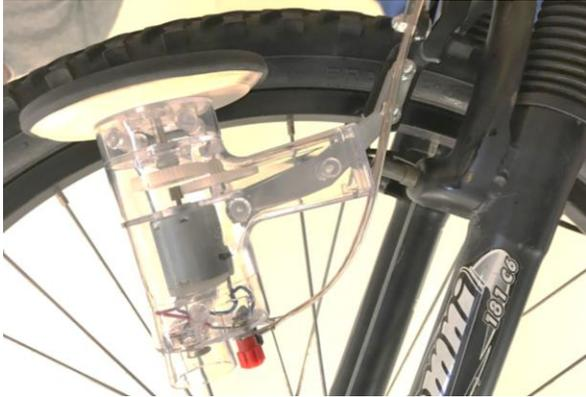
Figure 2a: RE-Brake attached to bike
