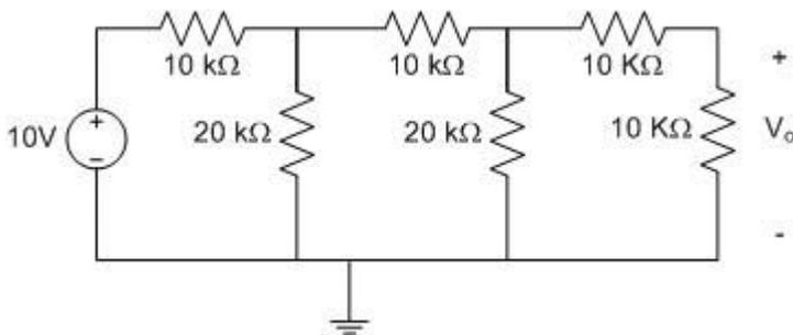
Figure 1. Circuit used to identify alternative methods for obtaining the output voltage.
