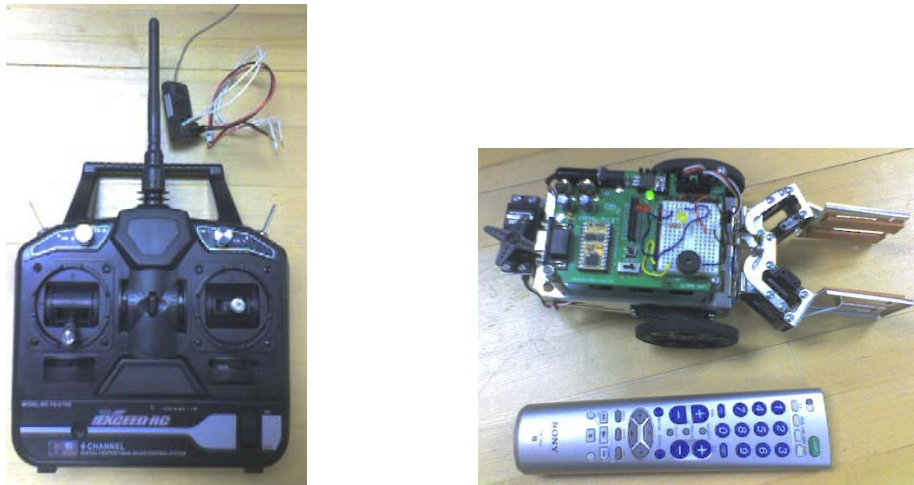
Figure 2: RC controller and BOE-Bot with TV Remote control
