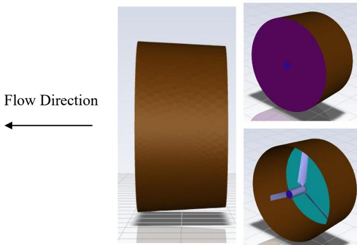
Figure 5: The images above depict the tapered shape of the fluid domain and the orientation of the turbine model within the domain.
