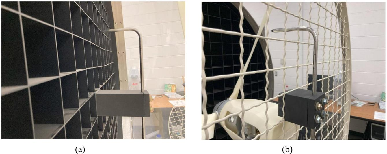
Figure 2: Pitot tube at the (a) upstream and (b) downstream locations.
