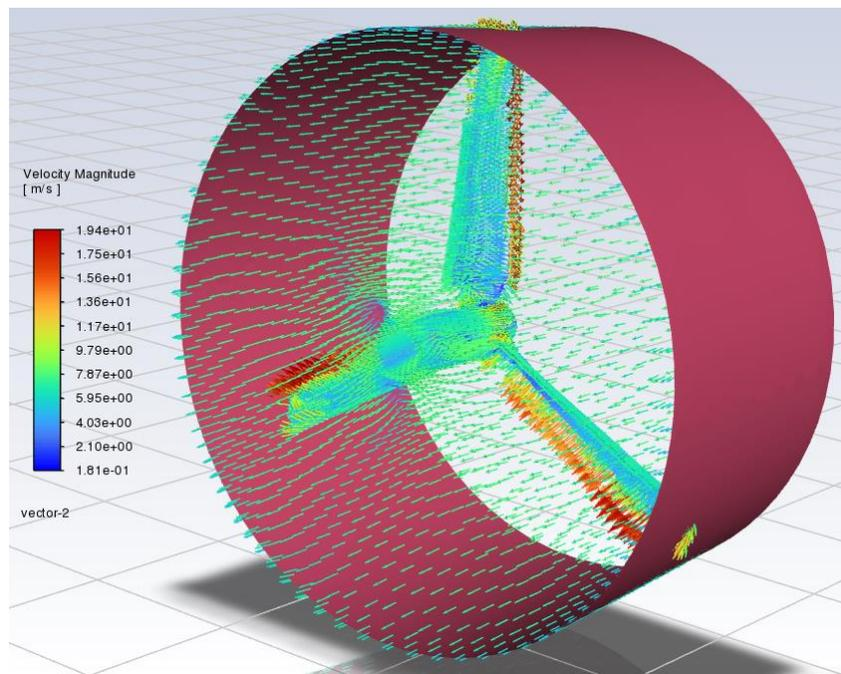
Figure 6 – Velocity field near the turbine blades.
