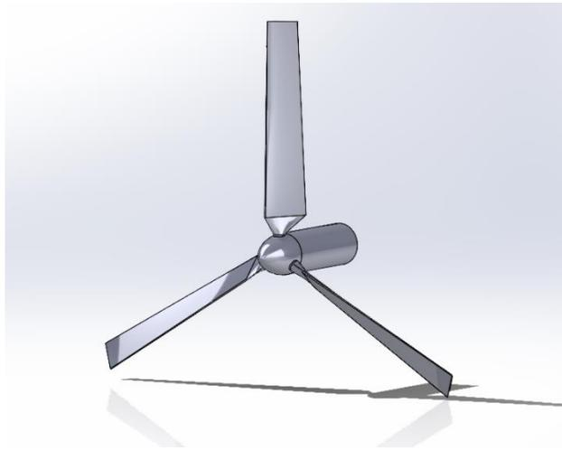
Figure 4: Computational model of the three-turbine blade geometry used in the CFD simulation.
