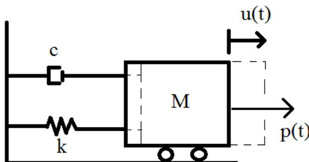
Figure 3. Mass-spring damper system.
