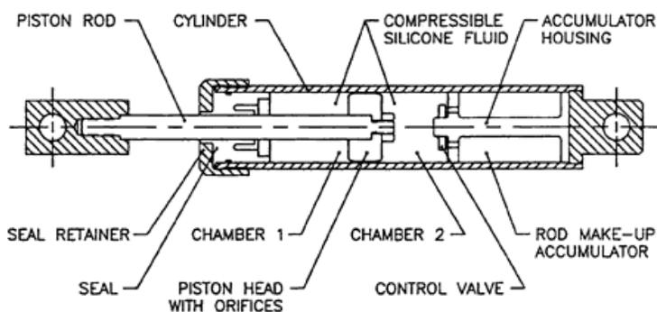
Figure 2. Fluid viscous damper<sup>2</sup>
