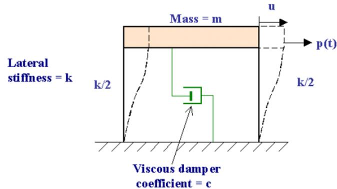
Figure 4. One story structure with damper<sup>6</sup>
