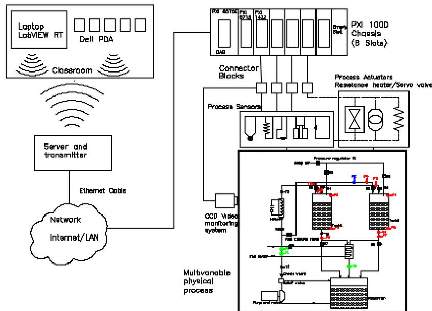
Figure 1: A multivariable process data acquisition and monitoring system
