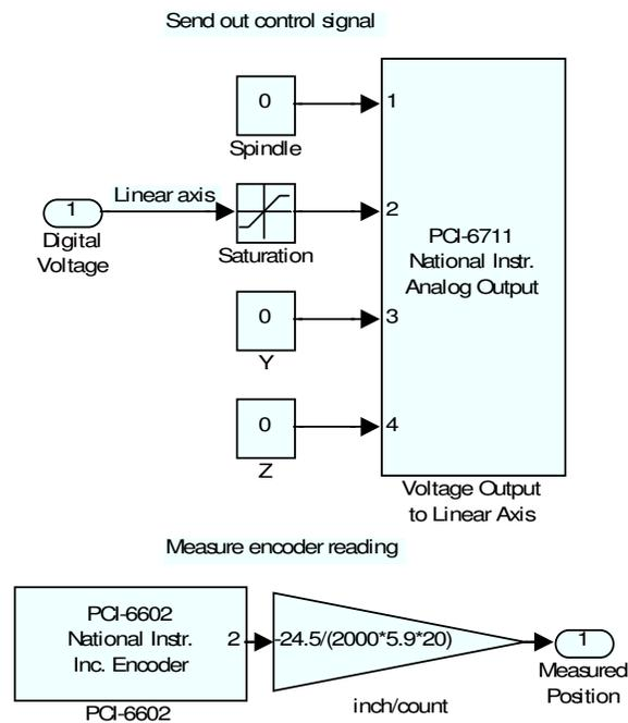
**Figure 7: Contents of Computer-System Interface for Implementation Mode.**
