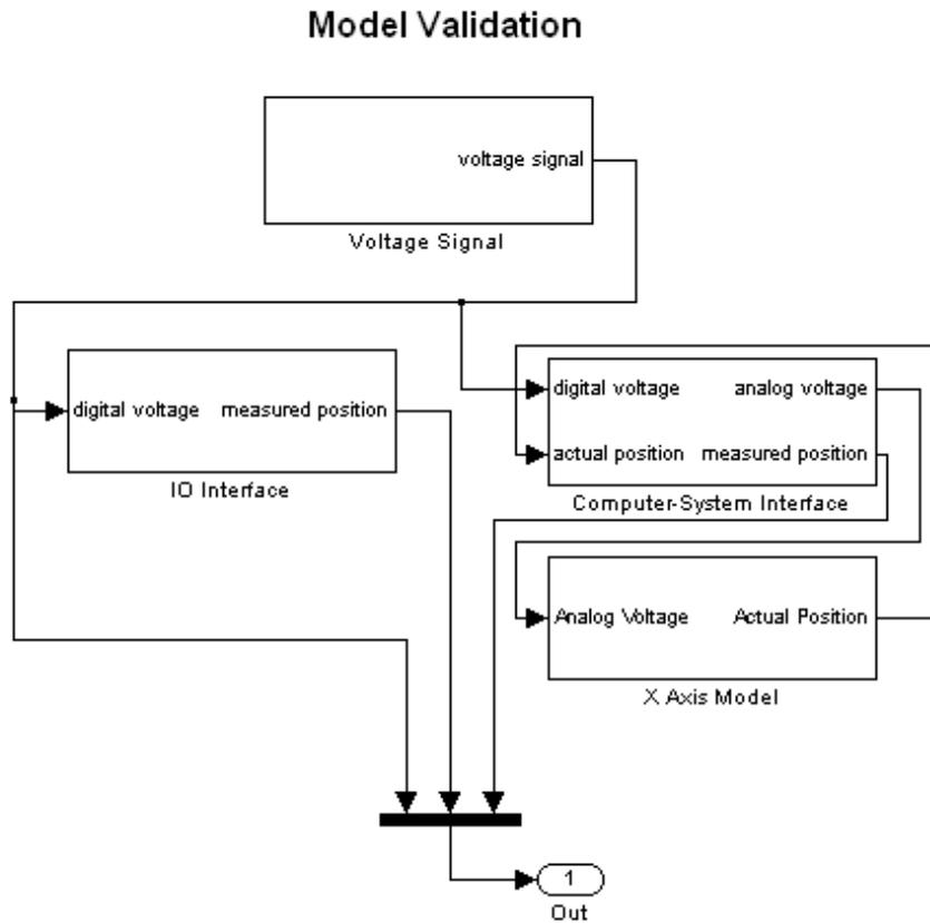
**Figure 10: Axis modeling model validation mode Simulink model.**
