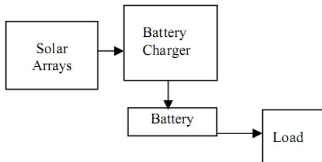
Figure 3: Implementation of photovoltaic power system.
