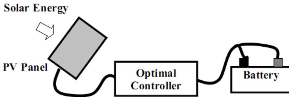
Figure 2: Schematic Diagram of a Solar Powered Battery Charger with Optimal Controller
