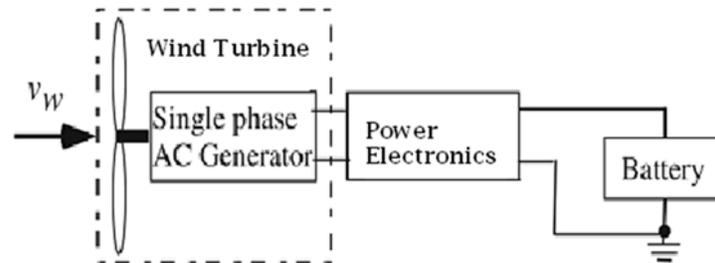
Figure 1: Physical Diagram of the Wind-Turbine-Battery System
