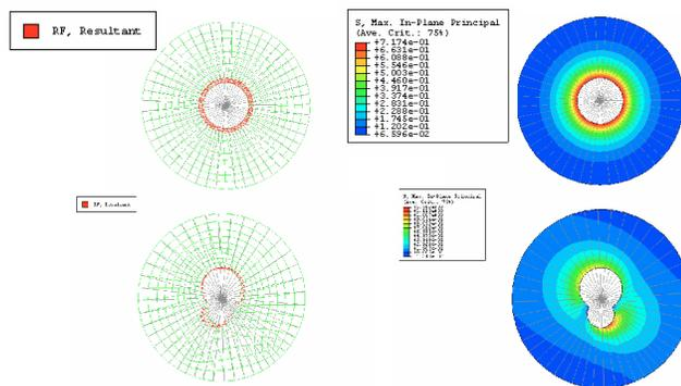
Figure 6: 2D Finite element modeling to study microscopic responses of each device's interaction with the bone
