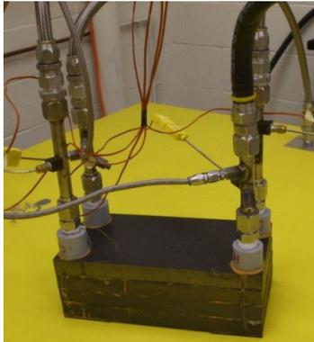
Figure 2: Cool polymer heat exchanger test setup.
