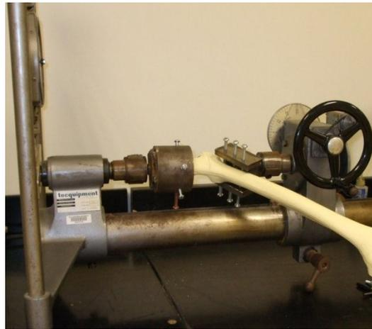
Figure 5: Torsion test to measure the relationship between applied angular rotation and the resultant torque
