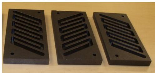
Figure 1: Prototype of cool polymer heat exchanger plates.
