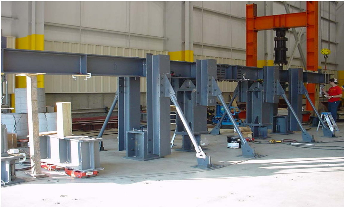
Figure 2. A View of the Test Set-Up Used for the Fuse Beam Testing
