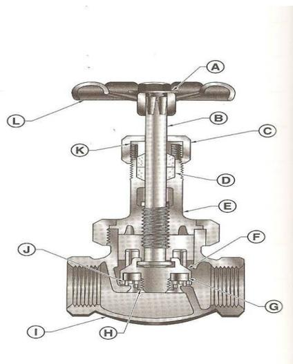
Figure 3: Components of a globe valve<sup>2</sup>
